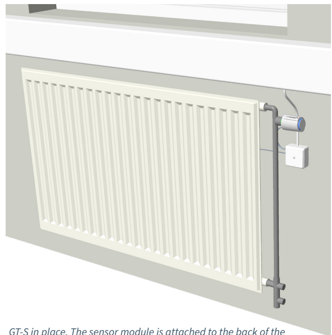
GT-S in place. The sensor module is attached to the back of the radiator, the valve actuator is mounted on the radiator valve, and the common connection box is attached to the wall with the four conductors to the room climate controller connected.
