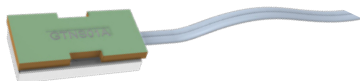
The sensor module (20x10x5 mm) consists of a smaller circuit board with a 2-conductor cable. The circuit board is mounted on a magnet that attaches the sensor to the radiator.
