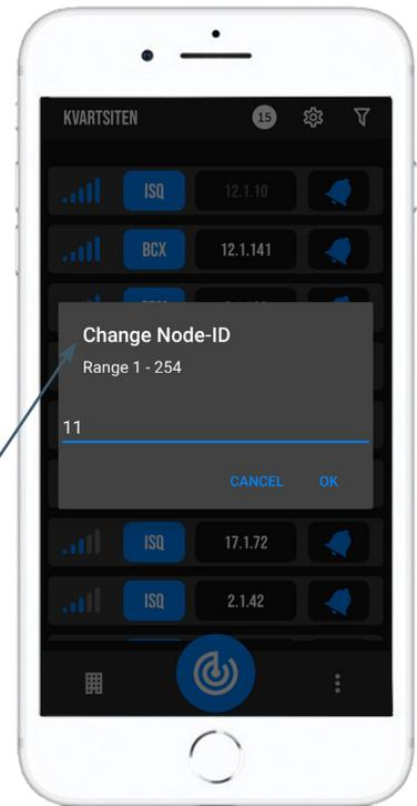
First Step in Commissioning: By selecting the Node-ID field for the intended device, a window opens where a new Node-ID can be set.
