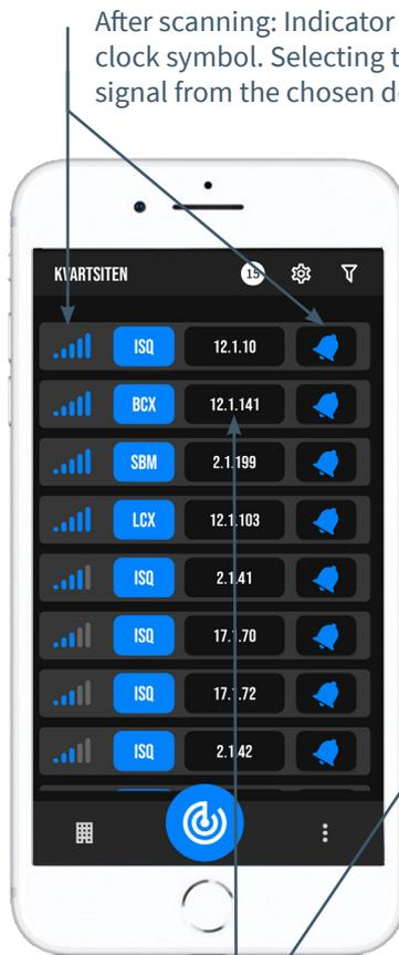
After scanning: Indicator for current signal strength and field with clock symbol. Selecting the clock symbol triggers an audio and light signal from the chosen device.
