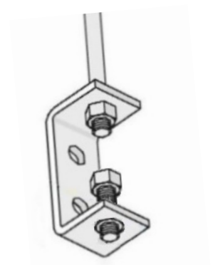
Example with a U-bracket as a suspension device. The bracket is mounted on the top of the plenum box with a screw (M8x16).
